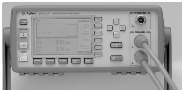
Figure 7. E4417A power meter configured to show a trace display (upper window) and a dual numeric display (lower window).
